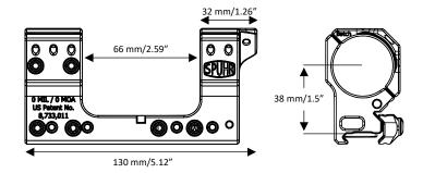
The mounts are machined from billet 7000 series aluminum and all aluminum parts are hardcoat anodized. The Torx 20 ring and clamping screws are zinc-nickel coated for corrosion resistance and come pre-waxed from the factory to ensure proper torque values.
