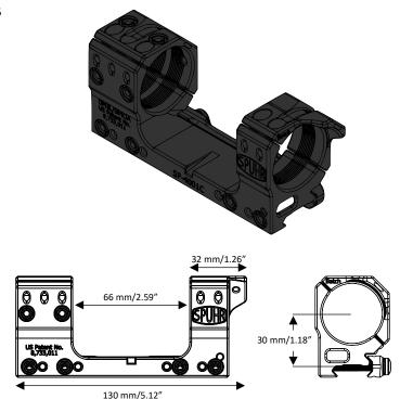
The mounts are machined from billet 7000 series aluminum and all aluminum parts are hardcoat anodized. The Torx 20 ring and clamping screws are zinc-nickel coated for corrosion resistance and come pre-waxed from the factory to ensure proper torque values.
