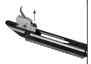
2. Unscrew the trigger bolt with the appropriate screw driver (typically a Hex 5) to remove the trigger (trigger safety on).
