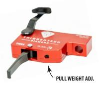
Your TriggerTech trigger is set near the middle of the advertised pull weight range and can be adjusted in increments. To adjust pull weight, insert the supplied 5/64" Allen wrench into the set screw located at the bottom of your trigger. To increase pull weight, rotate the set screw clockwise. Pull weight varies between actions.
