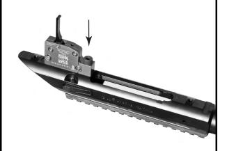
3. Insert the TriggerTech trigger assembly into the action with the trigger safety on. Using the same factory trigger bolt from Step 2. Tighten bolt to 55-65 in-lbs.
