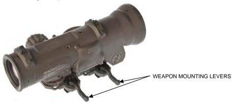
Figure 2-1: Levers lock sight to MIL-STD 1913 rail
